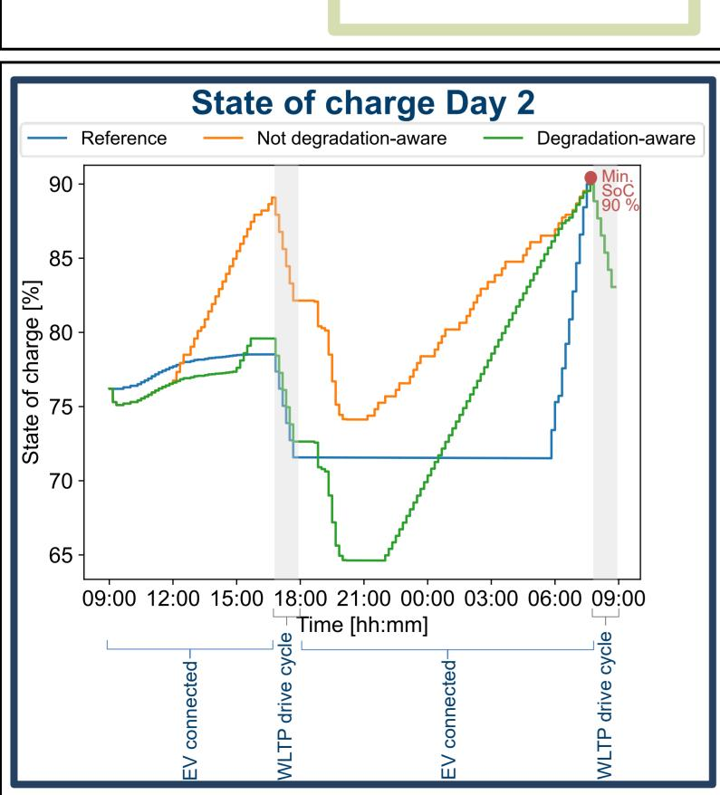
Day-Ahead scheduling **Objective Mixed-Inter Linear Program Electricity** Degradation **Grid charge** costs costs <sup>4</sup>  $c_t^{batt} = cycles_t \cdot \frac{c^{batt,invest}}{cycles^{max}} + c^{cal}(SOC_t)$ MILP models with variation in objective function and constraints: Not V2G-enabled, Reference: not degradation-aware V2G-enabled, Not degradation-aware: not degradation-aware V2G-enabled, **Degradation-aware:** degradation-aware
